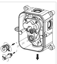
It is possible to open the outlet usually closed with a plug installing the diverter kit
